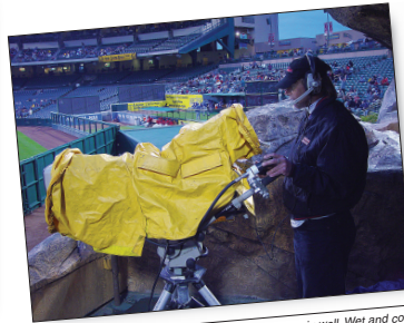
Figure 2.155 Water and electronics don't usually mix well. Wet and cold can conspire to fog the optics of the over $100K lens on the camera, as well as the prism and filters in the camera. Many lenses have internal heaters to prevent this problem.
